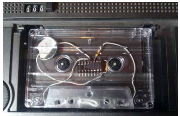
Fig. 1. The basic version of Programmable Tape set up in a traditional tape player.
