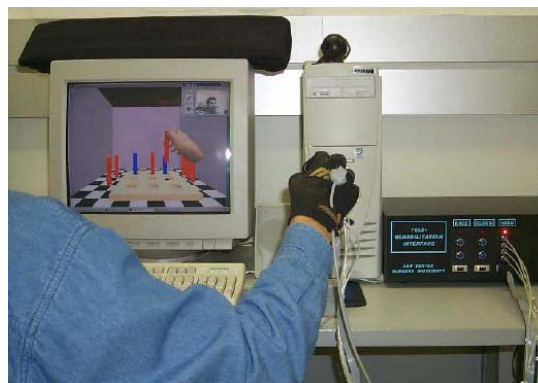
Figure 2. Rutgers Haptic Master being used to reflect grasp force during virtual chess match.
