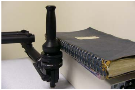
Figure 8. Detecting the rough edge of a spiral notebook during tele-assessment test.
