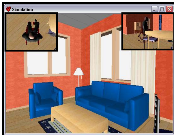
Figure 1. Screen shots of a typical HabiTest environment. The larger central view is the main view and is “first person” (ego-centric). Two additional auxiliary views are available – “bird’s eye” view (upper left corner) and “third person” side view (upper right corner). These views can be turned on and off as well as switched (i.e. the main view can be show bird’s eye point of view while the top right auxiliary view can show the ego-centric view).
