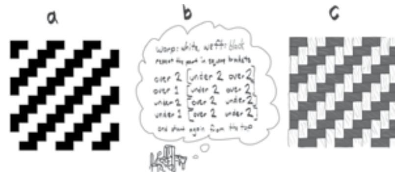
fig. 3: The digital image (a) is encoded as a set of weaving instructions by the weaver (b). These instructions are then decoded by the weaver back into a pixelated representation (c). The original pattern is thus digitally replicated. Automatic looms perform the (b>c) transition, and additionally store the representation of (b) in physical form: expert knowledge is only needed for encoding, and only once per pattern.
